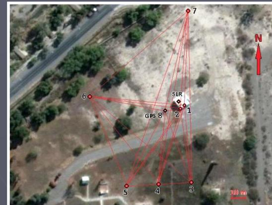
**Due to the impossibility of view between the terrestrial network points and mount SLR, we had to designing a particular methodology for connection**
